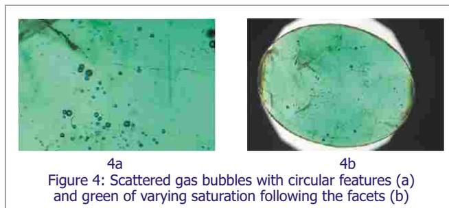
Figure 4: Scattered gas bubbles with circular features (a) and green of varying saturation following the facets (b)
