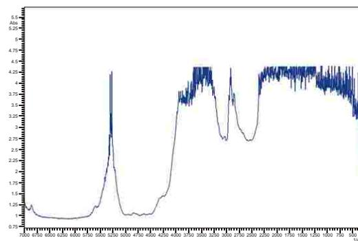
Figure 8: FTIR Spectrum of these new composites is consistent with that of a natural beryl
