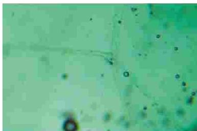
Figure 6: Yellowish junction between the layers due to glue
