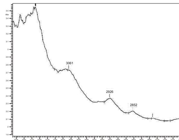
Figure 15: Typical FTIR spectrum of polymer-filled tanzanite
