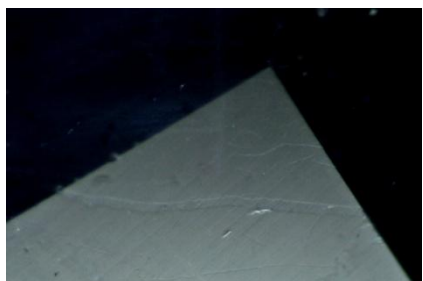
Figure 2.a: Under reflected light, glass-filled fractures appear as dull lines, due to low hardness of filler glass.
