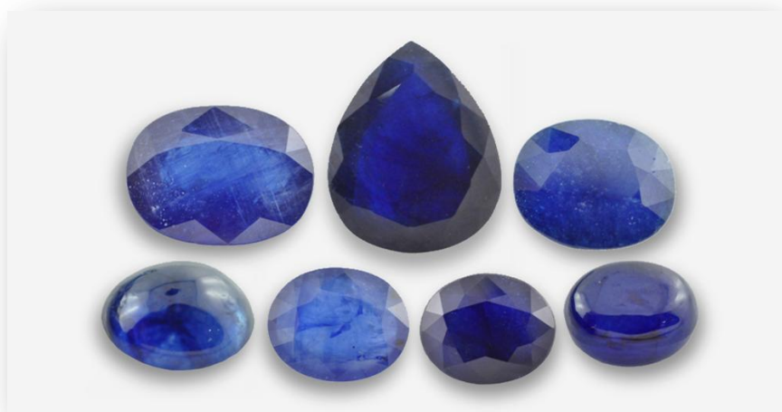
Figure 1: Representative samples of cobalt coloured lead-glass filled sapphires received at the Gem Testing Laboratory, Jaipur for identification
